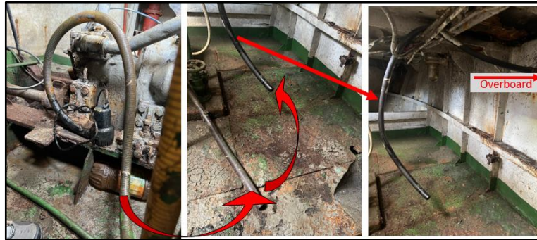
Figure 12 - View of the disconnected bilge pipe inside engine compartment of YM3 ( Source: the TSIB )
