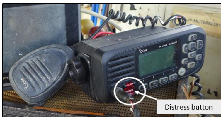
Figure 1 – One of the three VHF sets inside the wheelhouse with annotation of the distress button ( Source: the TSIB )
