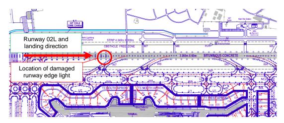
Figure 1. Location of damaged runway edge light
