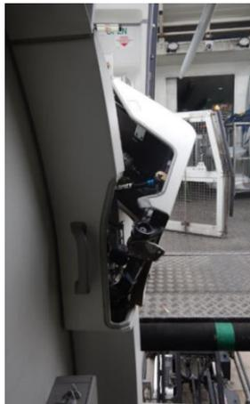
Figure 5: Damage to the door hinge
