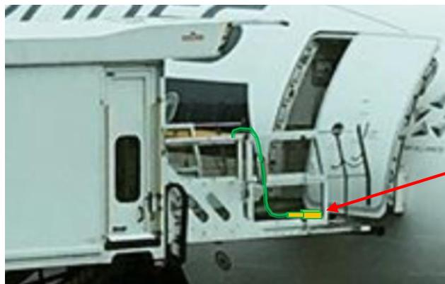
Safety shoe placed between aircraft door and truck cabin platform
