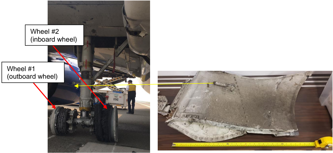
Figure 1: Damage to the left landing gear (left photo, view from the rear of aircraft) and the left landing gear panel retrieved from Changi Airport (right photo)
