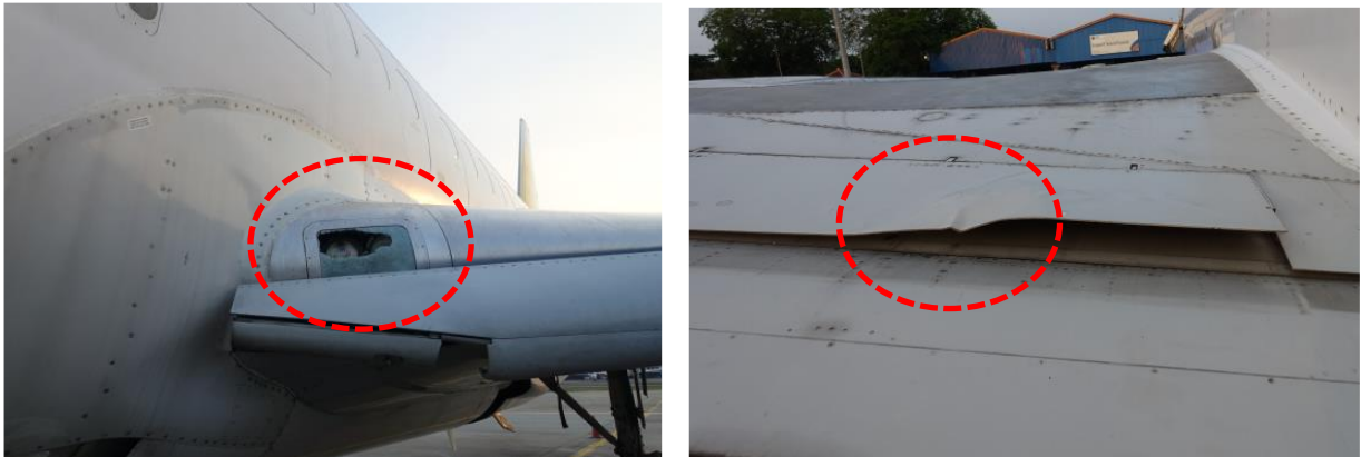
Figure 3: The left landing light was damaged (left photo) and trailing edge of left wing was deformed (right photo)
