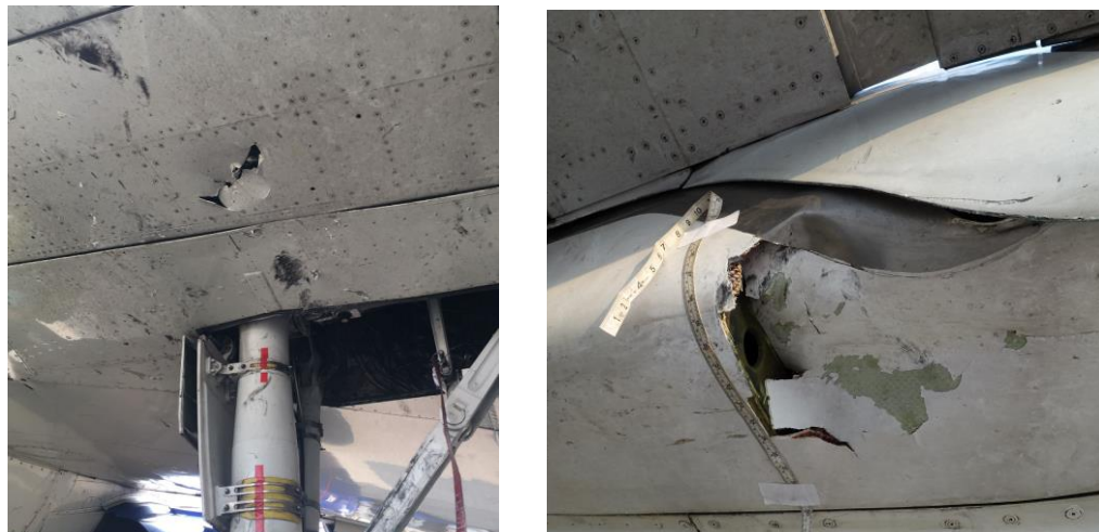
Figure 2: Damage to the underside of the left wing
