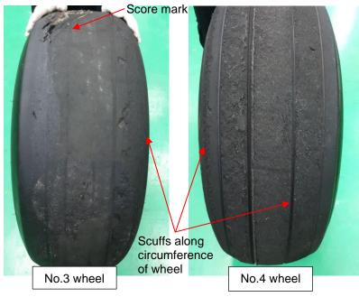
Figure 6: Damage on tyres of RH MLG
