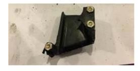
Figure 4: Hydraulic line guide
