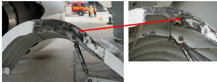
Figure 3 – Damaged frame on fixed door of left MLG
