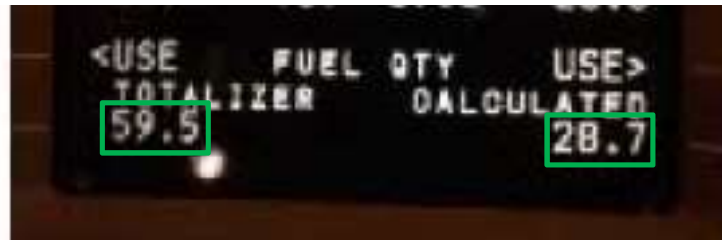
Figure 5. FMC displaying the discrepancy between “measured fuel” remaining (i.e. totalizer) and “calculated fuel” remaining (i.e. calculated)
