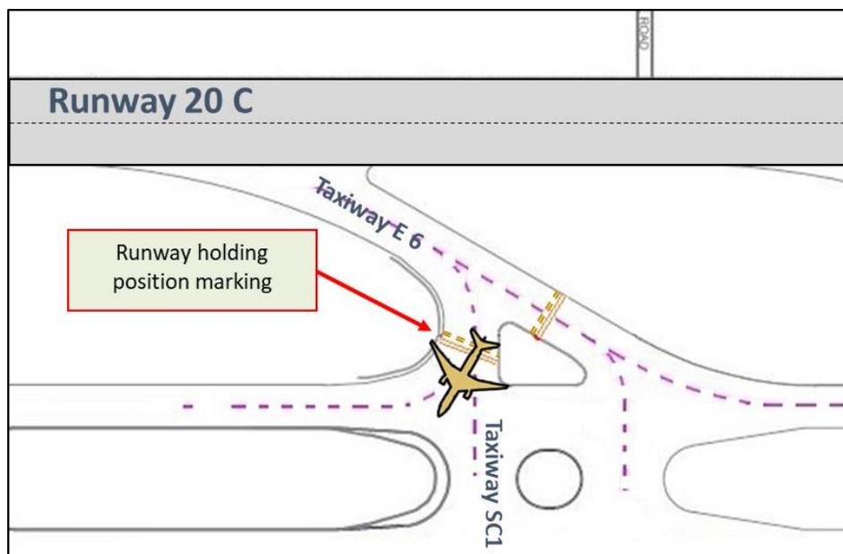
Figure 4. Orientation of B777 at E6
