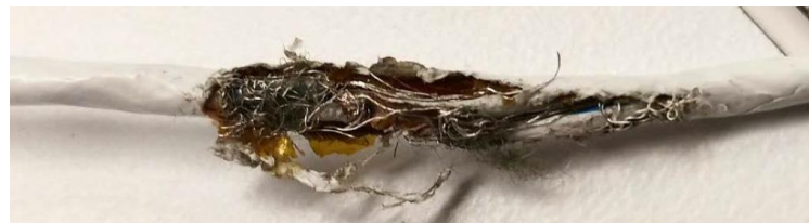
Figure 5: Damaged wire and cable insulation found
