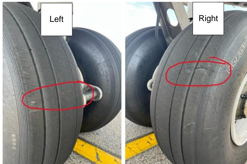
Figure 4: Damage on each nose wheel
