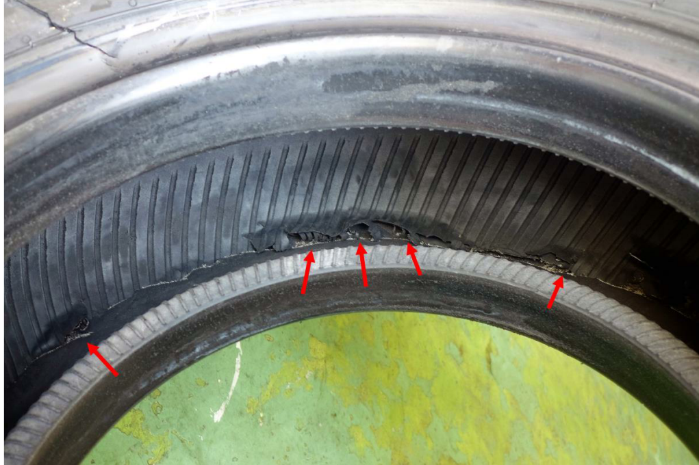
Figure 6: Continuous crack line along the interior shoulders of the tyre
