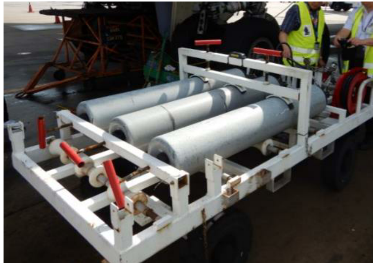
Figure 3: N 2 servicing cart
