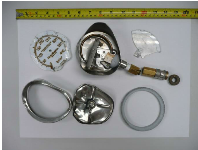
Figure 4: Shattered manual tyre pressure gauge
