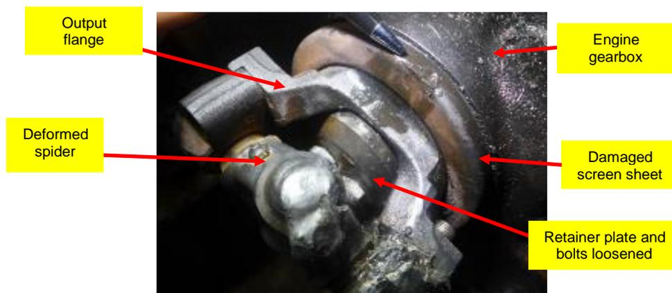
Figure 16: Deformed spider of universal joint
