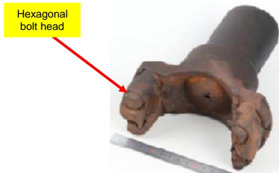
Figure 19: Hexagonal bolt heads on the fixed yoke of the cleaned-up transmission shaft assembly
