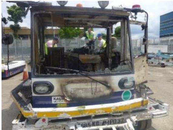
Figure 3: Damage to the driver's cabin of the tow tug
