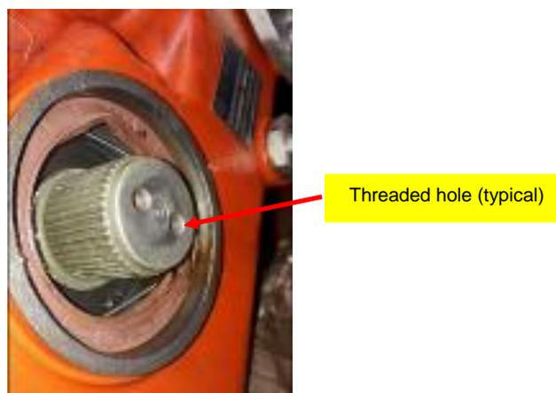
Figure 15: Output shaft of the engine gear box (output flange removed for clarity)
