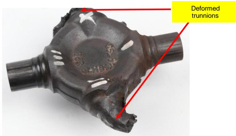
Figure 14: Damaged spider of the universal joint connected to the output flange
