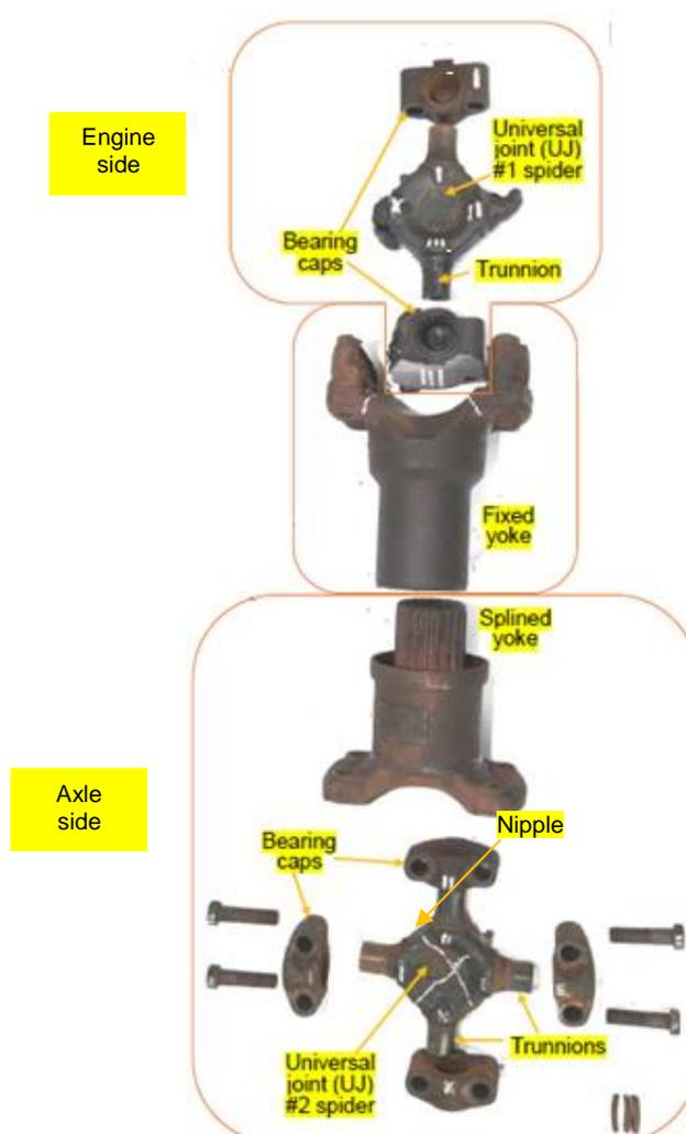
Figure 7: Transmission shaft assembly
