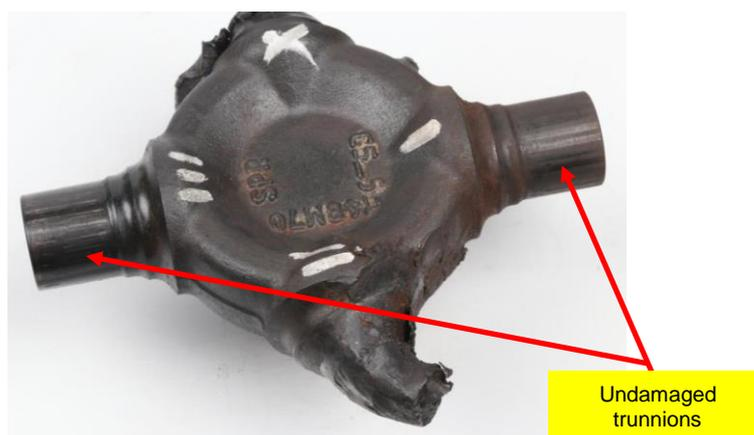
Figure 17: Undamaged trunnions
