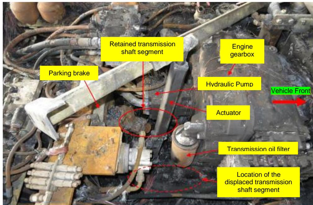
Figure 11: Damage to components under the engine hood
