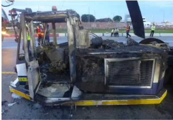
Figure 5: Damage to the left side of the tow tug
