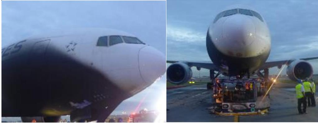
Figure 2: Damage to aircraft structure and nose landing gear
