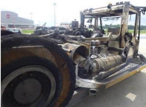
Figure 4: Damage to the right side of the tow tug
