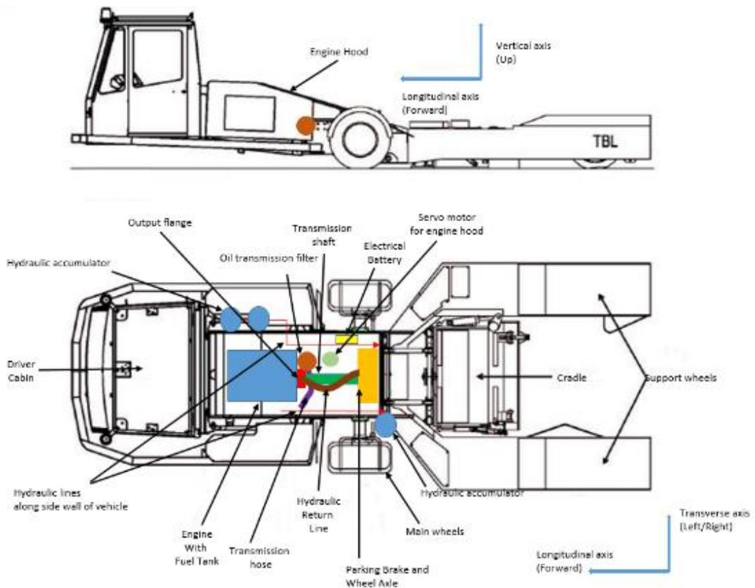
Figure 6: Tow tug schematic
