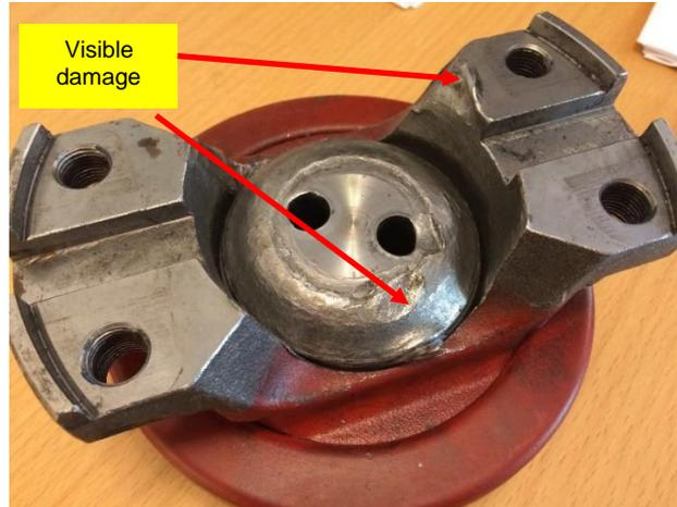
Figure 18: Damage on output flange and retainer plate
