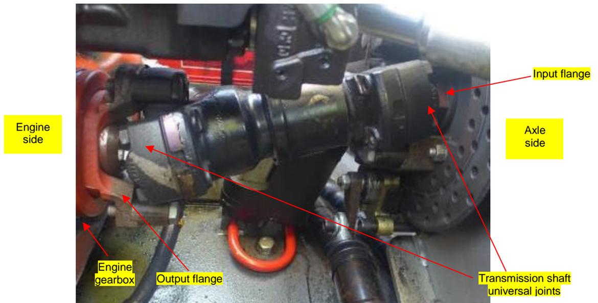
Figure 8: Transmission shaft assembly in situ
