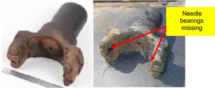
Figure 13: Fixed yoke segment of the transmission shaft assembly (left photo showing the component after cleaned-up)
