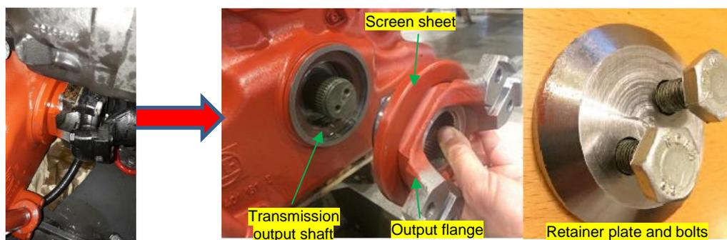
Figure 9: Retainer plate holding output flange (illustration picture only)
