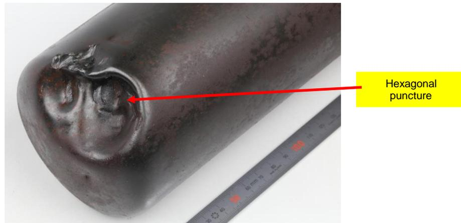
Figure 20: Hexagonal shaped puncture on the transmission oil filter casing
