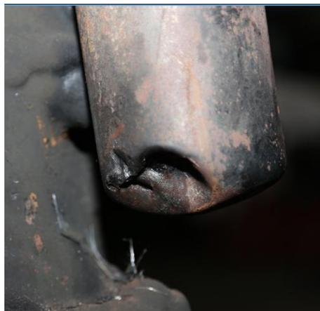
Figure 12: Puncture on the underside of the transmission oil filter casing
