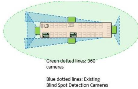
Images showing how the 360-degree collision warning system would enhance safety (for illustration purposes only)
