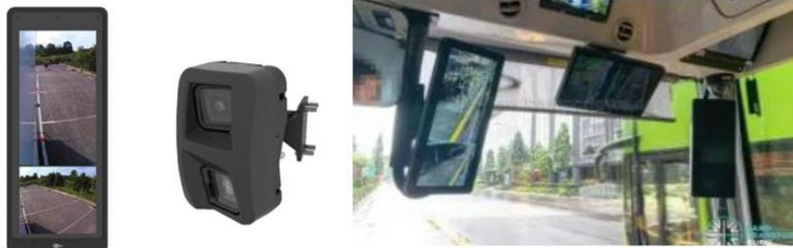
Images showing the camera mirror system being trialled on a bus (for illustration purposes only)
