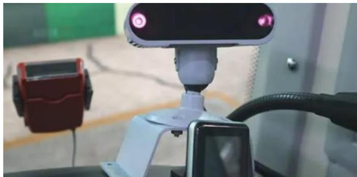
Image showing the anti-fatigue system installed on a bus (for illustration purposes only)
