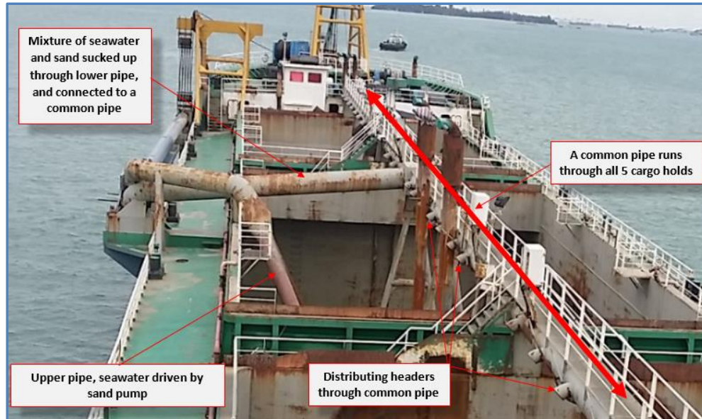
Figure 10 – Layout of suction system on CJ2 (CJ3's was similar)
