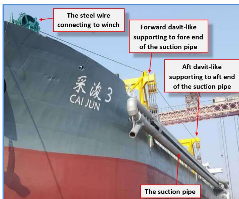
Figure 7 – CJ3's suction pipe, two davit supports and winch wires (Source: ISM Manager)
