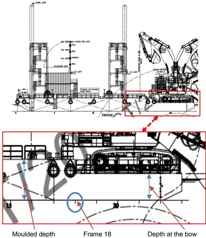
Figure 16 – Indicating the bow with depth at the bow (*Source: the Operator – Starboard side profile view of CB GA Plan, annotated by the TSIB*)
