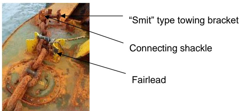
Figure 17 – “Smit” type towing bracket on the forward starboard bow (*Source: the Operator – annotated by the TSIB*)
