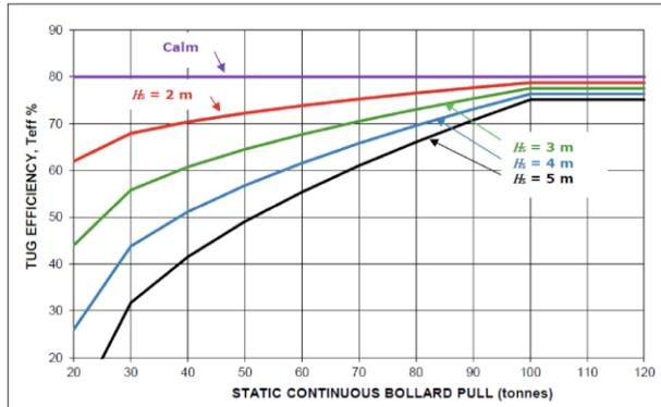
Figure 26 – Tug efficiency graph (Source: DNV-ST-N001<sup>59</sup>)
