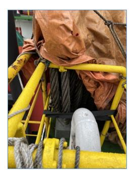
Figure 22 – Wire rope covered with canvas (Source: the TSIB)
