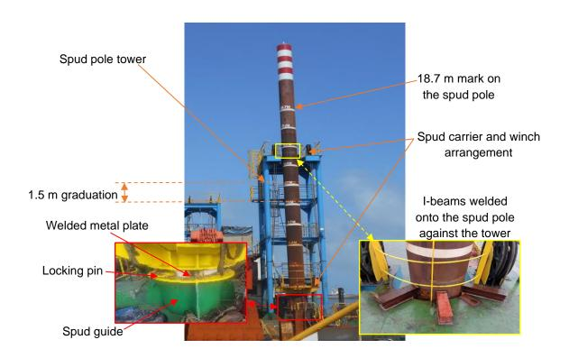
Figure 25 – Description of spud pole (*Source:* Operator – annotated by the TSIB)
