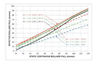
Figure 27 – Effective bollard pull graph (Source: DNV-ST-N001)
