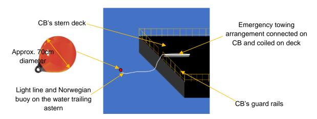
Figure 20 – The Norwegian buoy and the light line from CB (Source: the Operator – not to scale - For illustration only)
