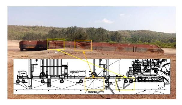
Figure 13 – Heavy indentation found on CB's starboard hull in way of Frames 11 to 13 and 16 to 18 – see annotation on General Arrangement (GA) Plan (Source: the P&I Club)
