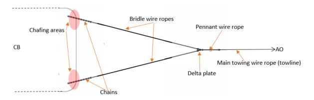
Figure 18 – Towing arrangement (not to scale) (Source: the Operator – annotated by the TSIB)
