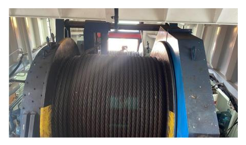
Figure 21 – Main towing wire rope on the main towing winch drum (*Source:* AO)
