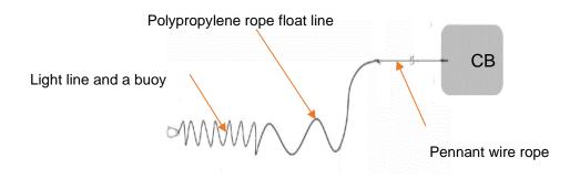
Figure 19 – The emergency towing arrangement on CB (Source: the Operator – not to scale)
