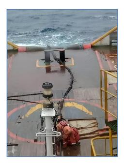
Figure 6 – The damaged towing pennant wire rope showing unravelled strands (*Source:* the Operator)
