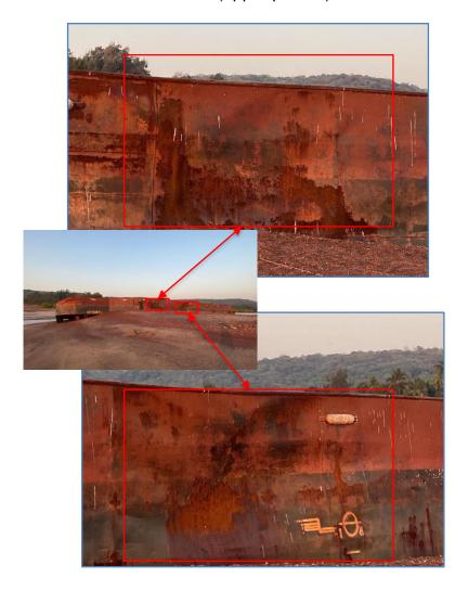
Figure 12 – Indentation on CB's starboard hull (Source: the Operator)
