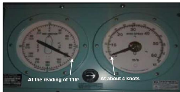
Figure 8 – Wind direction & speed shown on the wind indicator at 0400H, 1 June 2022 (Source: the Company, annotated in white by the TSIB)
