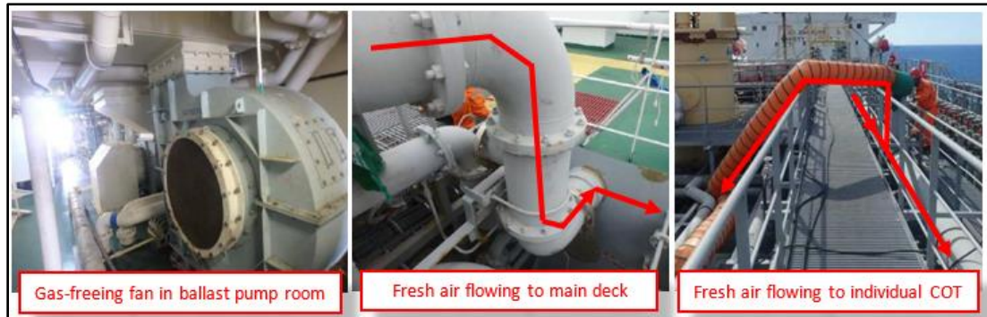
Figure 5 – Flow of fresh air driven into the individual COT from the fixed gas-freeing fan (red annotated by the TSIB; Source: the Company)
