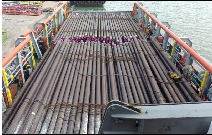
Figure 8 – View of the casing bundles stowed onboard the Nautla (Source: the Company)
