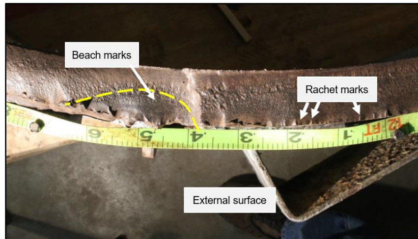
Figure 9b – Presence of the beach and ratchet marks on the fracture surface of the pedestal ( Source: the laboratory's metallurgical analysis report )
