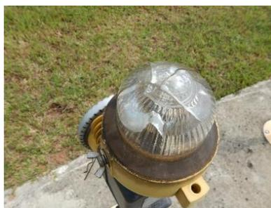
Figure 2. Approach light with broken top cover
