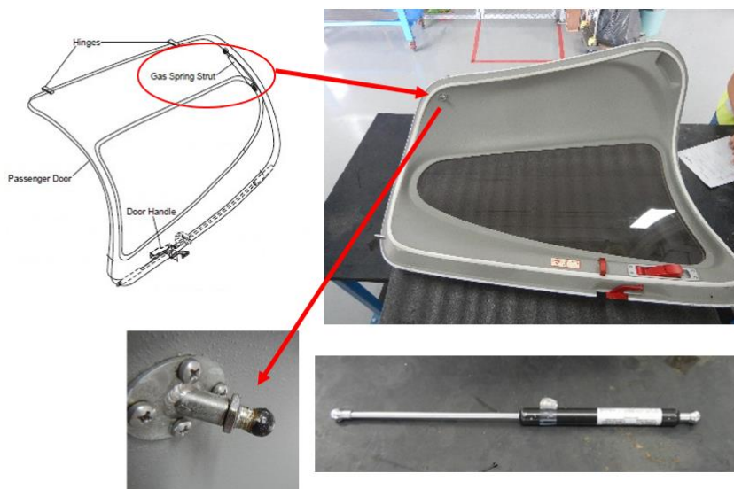
Figure 5. Gas spring strut detached from the door
