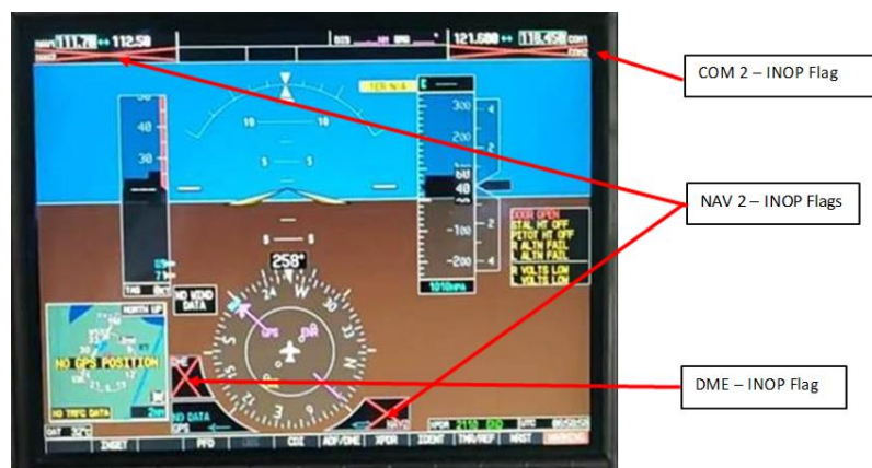
Figure 11. INOP flags on the PFD when the AMS is not switched on
