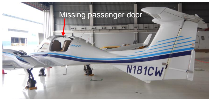
Figure 1. Passenger door detached from aircraft
