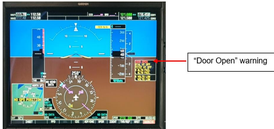
Figure 10. "Door Open" warning on the PFD
