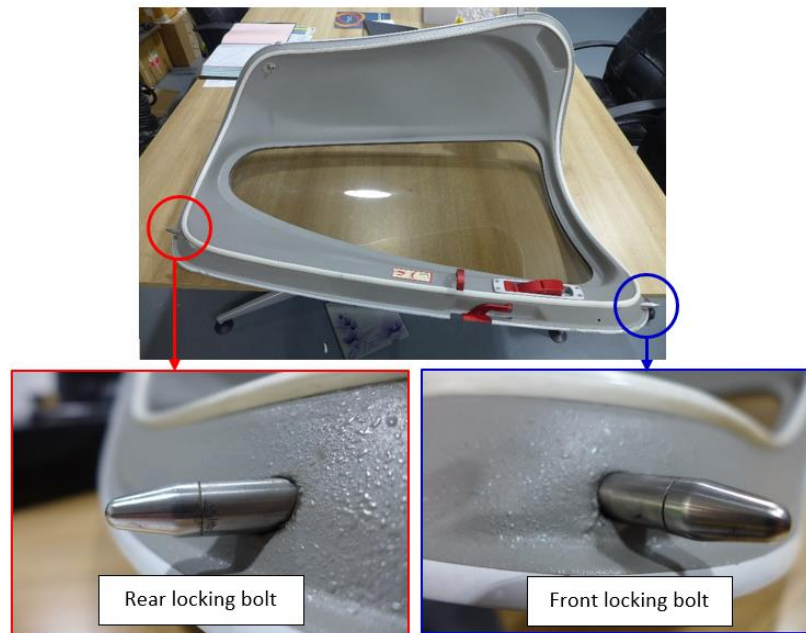
Figure 8. No damage on the locking bolts
