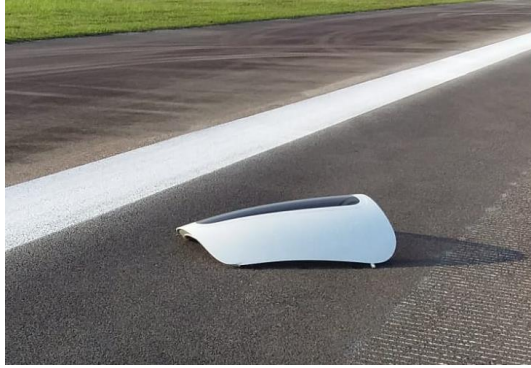
Figure 2. Detached door found on the runway
