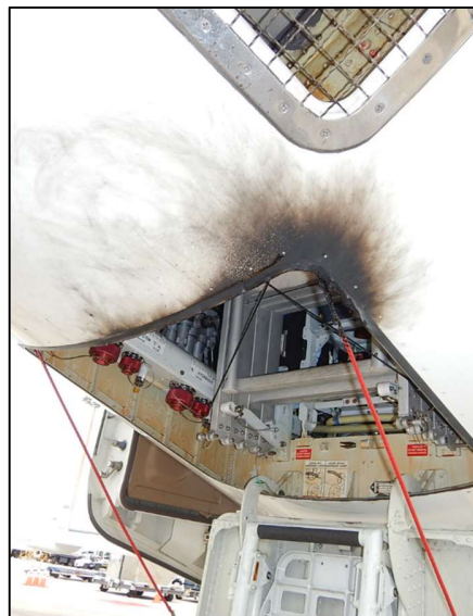
Figure 2: Damage to mechanic service compartment
