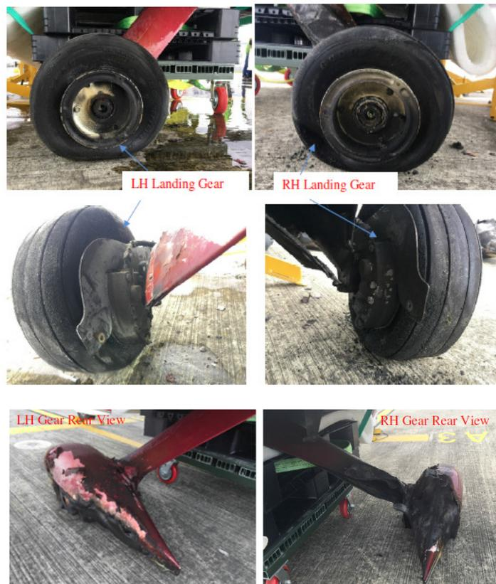
Figure 4: Damage to the landing gears
