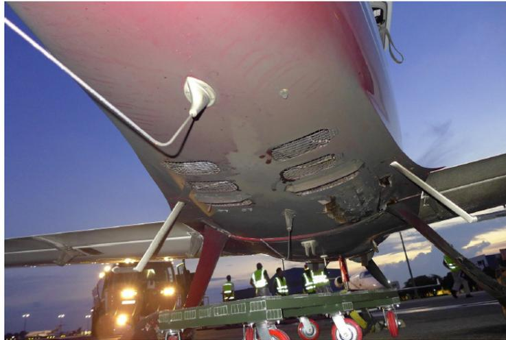
Figure 5: Heat damage on the lower fuselage of aircraft
