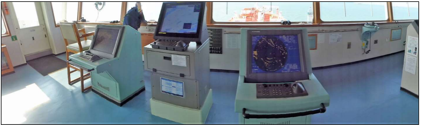
Figure 2 – AM's Bridge layout, indicating the X-Band ARPA (left), ECDIS (center) and S-Band ARPA (right)
