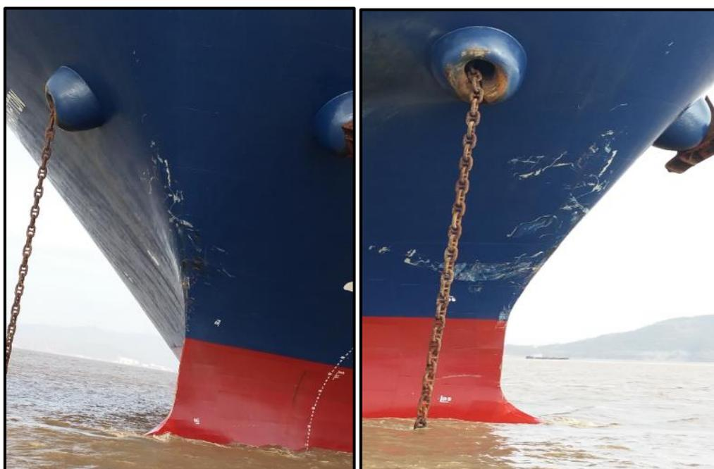
**Figure 5:** Paint scratch marks and minor indentations on the forward hull, above waterline.
