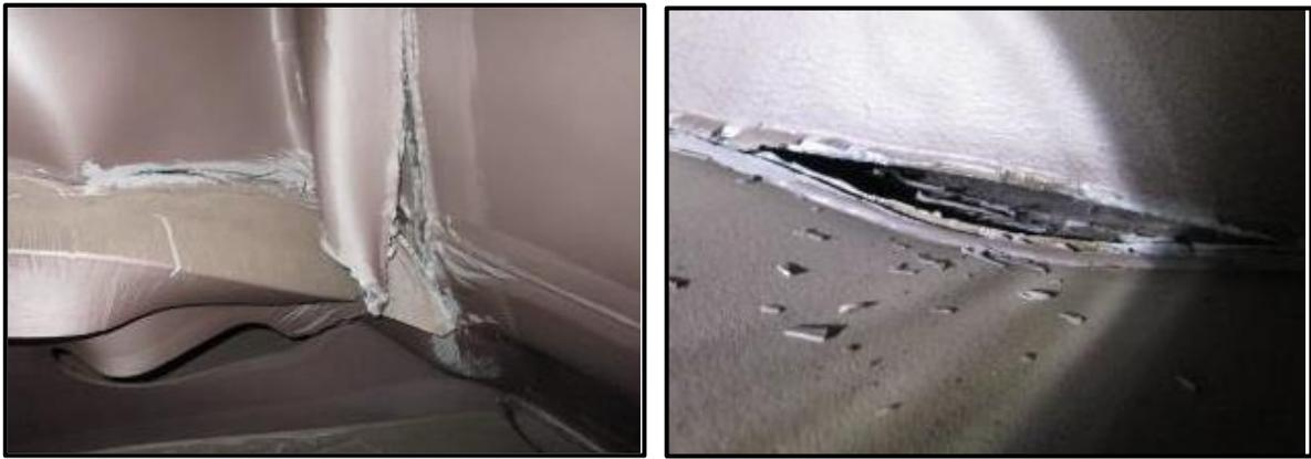
**Figure 6:** Buckled frames and fractured welding seams on the port side to forward of the bulbous bow (*Photo source: ISM Manager*)
