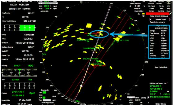
**Figure 1**: X-band radar acquired the presence and identity of fishing vessel ZLY annotated in blue by TSIB, and other vessels in APLS' route at about 2313H.
