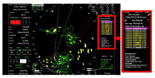
Figure 8: AIS broadcast messages on APLS' S-band radar display
