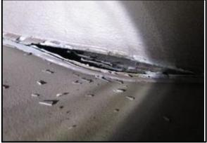
**Figure 6**: Buckled frames and fractured welding seams on the port side to forward of the bulbous bow (*Photo source*: ISM Manager)
