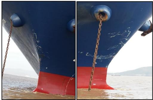
**Figure 5**: Paint scratch marks and minor indentations on the forward hull, above waterline.
