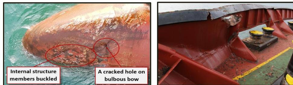
Figure 10 – Damage at ship bow areas after the collision
