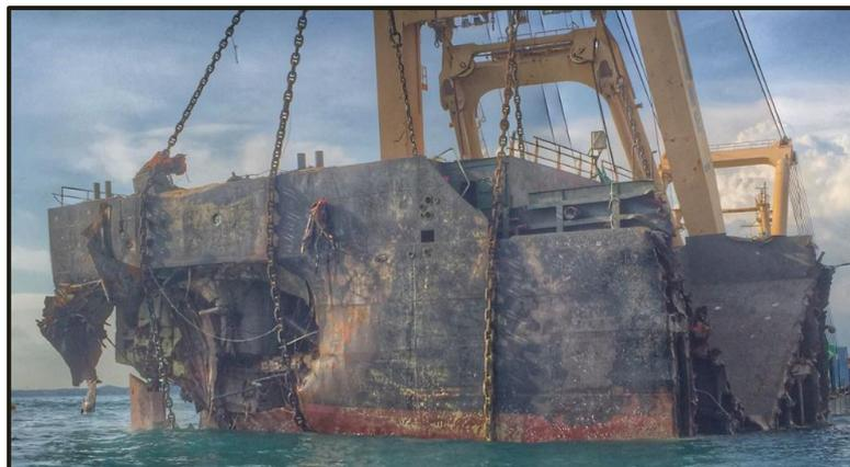
Figure 9 - The starboard quarter of JDR 19 being lifted out of water showing the angle and location of impact from KS's bow.
