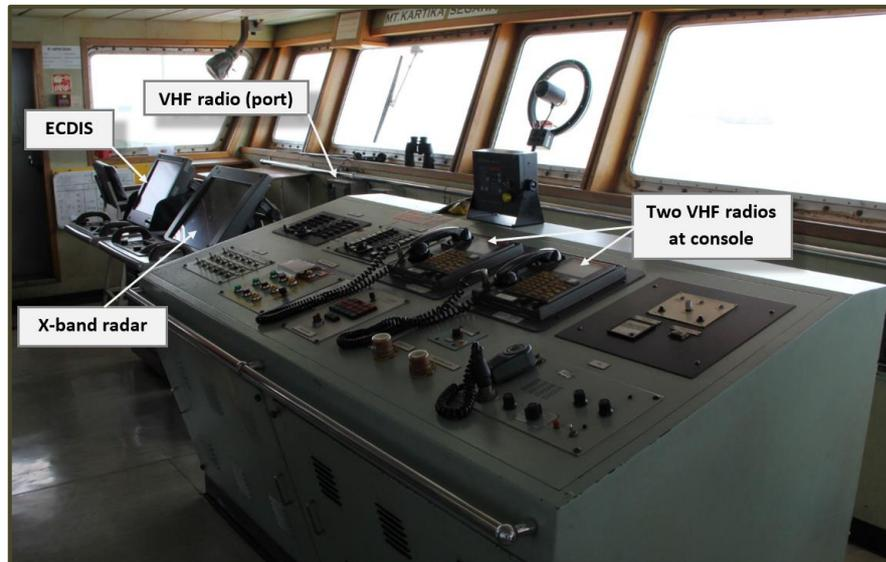
Figure 13 – Bridge equipment locations on KS
