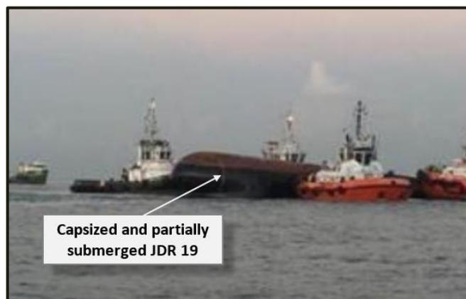
Figure 8 - Capsized and partially submerged JDR 19 was towed by four tugs
