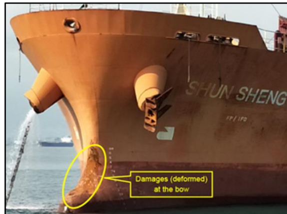
Figure 25 – SS' condition with damaged bow ( Source: TSIB )
