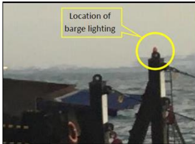
Figure 17 - Close-up view of Koi 5's forward section showing the "Red Light" (Source: MPA)
