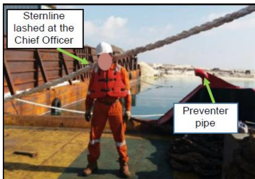
Fig. 6 – Stern line slipped out from the preventer pipe
