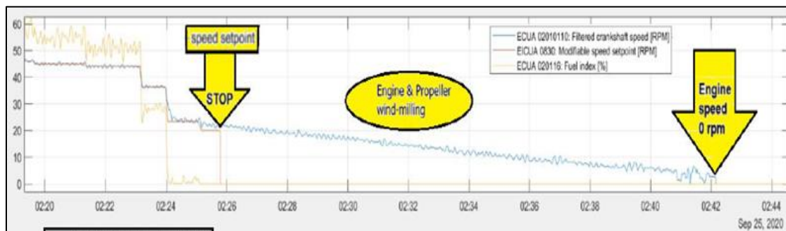
Figure 6b: Graphical representation of Line recorder extract showing speed setpoint stopped, engine & propeller wind-milling 37 until 0243H (i.e. when engine RPM comes down to Zero) - (Source: The ED)
