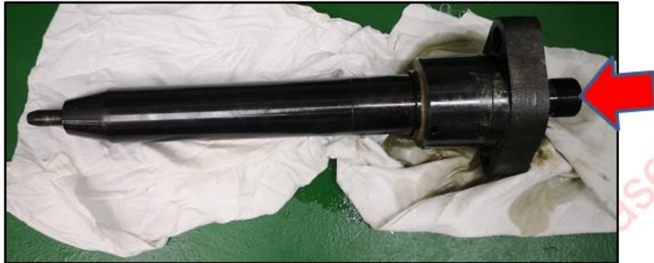
Figure 3: The FOIV from the no.4 cylinder of the main engine. (annotated by TSIB) Source: Engine crew of YSH.
