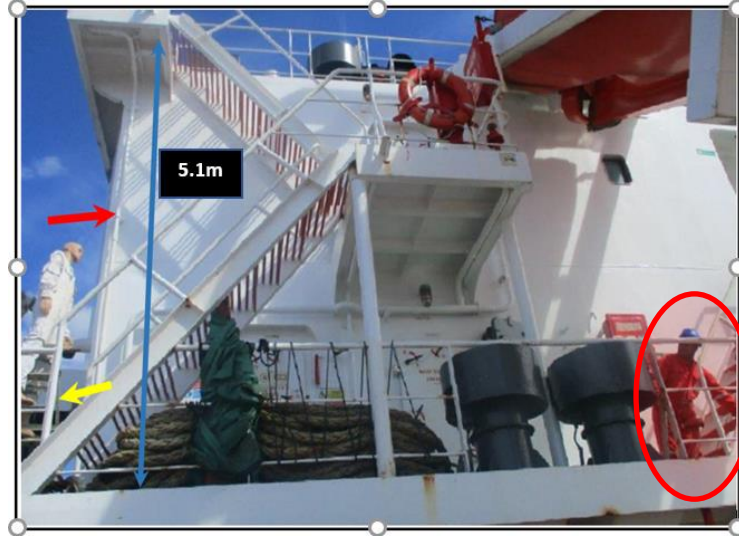
Figure 7: Viewed from the stern, depiction of the erected A-frame ladder's position (yellow arrow) on the portside of the boat-deck. Red arrow points to the drainage pipe. ASD-1's (circled in red) back was facing the ASD-3.
