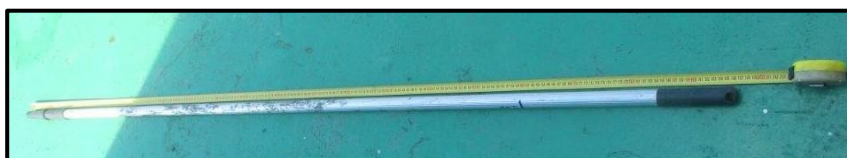
Figure 2: One of the telescopic rods used for the painting job by the ASDs. The rod was about 5m in length when fully extended.
