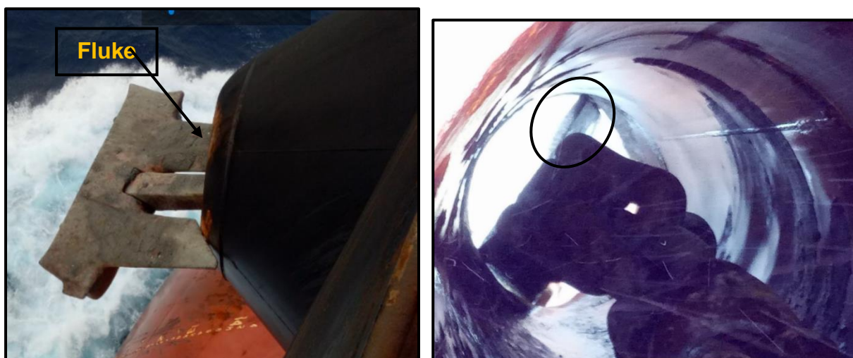
Figure 1: One of the flukes of the port anchor stuck inside the hawse pipe (Image on the right fluke viewed from inside the hawse pipe)
