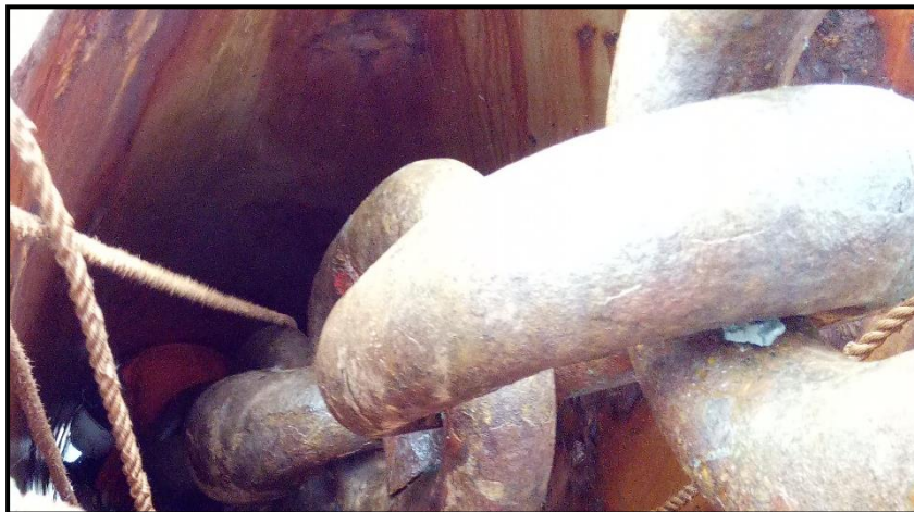
Figure 4: Bosun trapped between the anchor chain and the upper part of the hawse pipe
