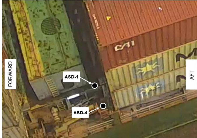
Figure 1 - Image captured by the terminal crane's CCTV showing the position of the two ASDs at about 0302h.
