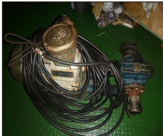
Figure 1 – Portable pump intended to be used for sludge discharging (Photo source: the ISM Manager)
