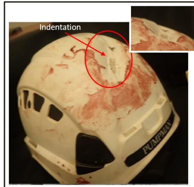
Figure 5 - the indentation of the Pumpman's helmet, viewed from two angles (Source: the ISM Manager)
