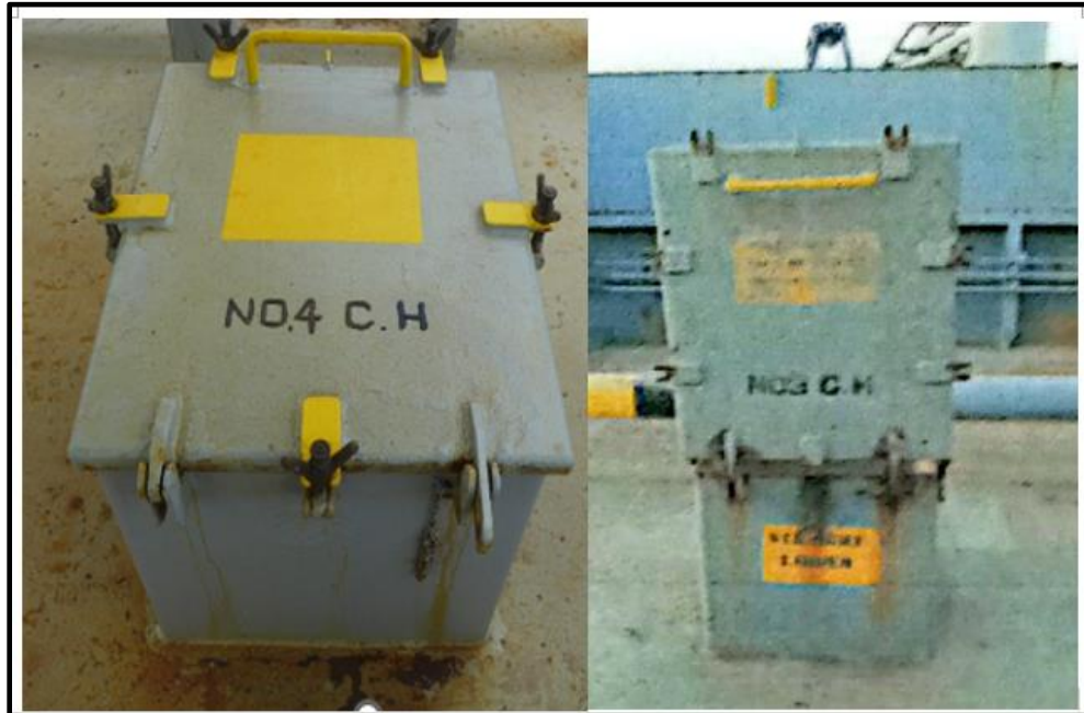
Figure 3: The left picture shows the (incomplete) painted top surface of the booby hatch cover, aft of CH4, after the welding maintenance work was completed at an earlier date. The right picture (provided by the Company) shows the original, pre-maintenance condition of the booby hatch, aft of CH3.
