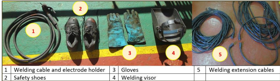
Figure 7 – Welding cables and PPE reportedly used by the Welder (Source: The Company)
