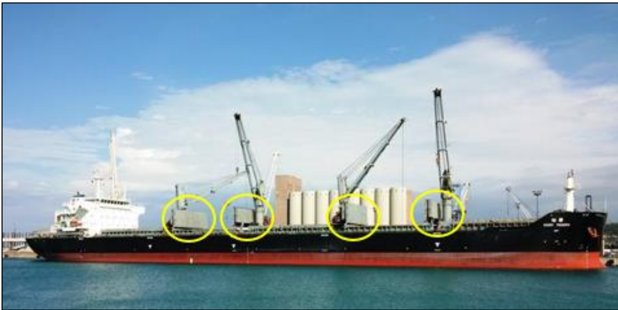
Figure 2 - Asian Triumph with hatch covers in open position as circled in yellow. Annotation by TSIB (Source: Marine Traffic)
