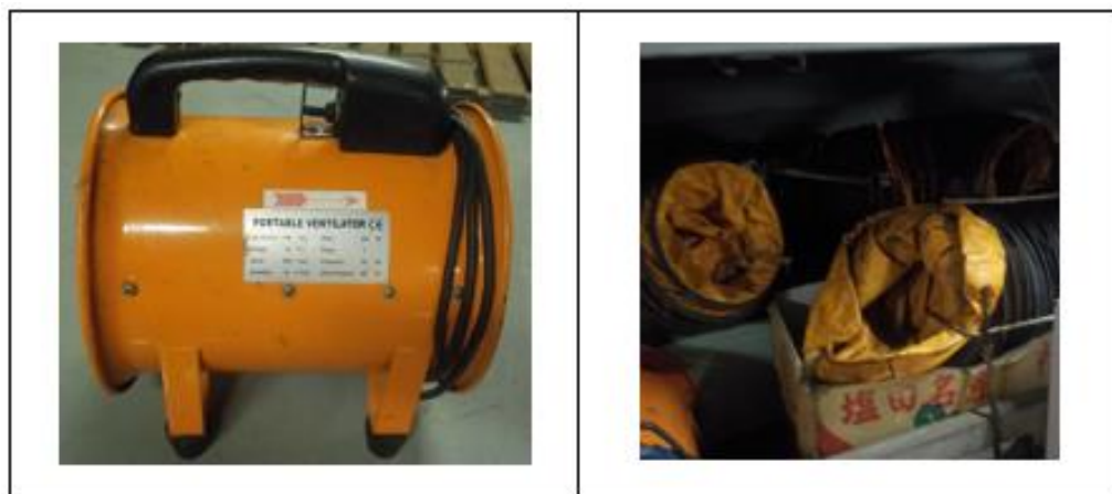
Figure 14 - The onboard portable fan and ventilation tubing. Source: The Company
