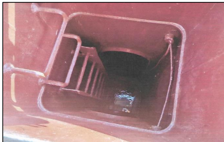
Figure 12 - showing the vertical ladder to the transverse beam walkway space. Source: The Company.
