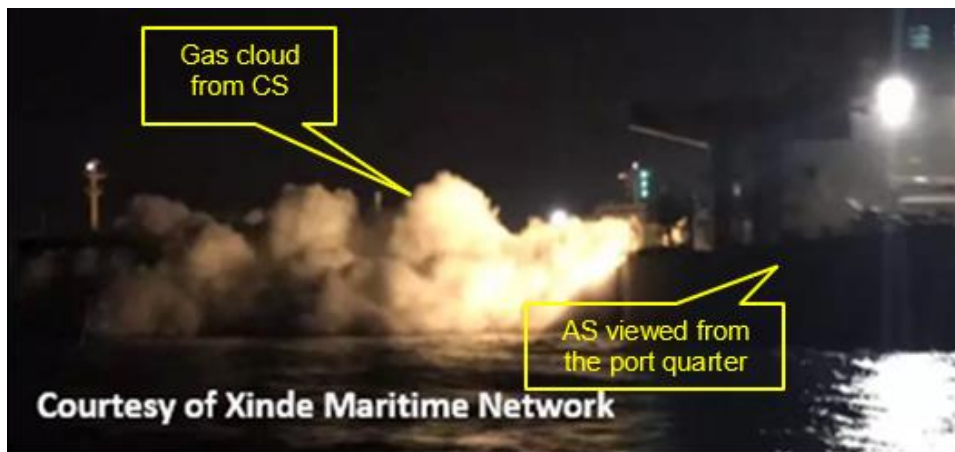
Figure 10 – Showing cargo leakage from CS into the atmosphere
