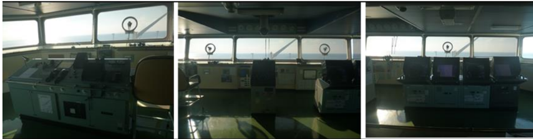
Figure 28 - From left to right – Telegraph console, steering column (with RoT indicator) and radar/ECDIS consoles
