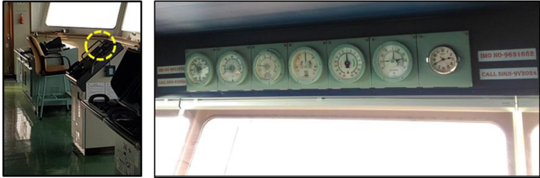
Figure 29 - Panel above the conning position showing, among others, wind speed and direction, engine rpm, rudder angle, etc.
