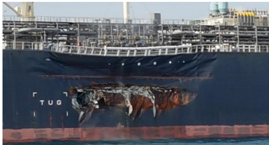
Figure 11 - External view of the vessel's damages in the midship section
