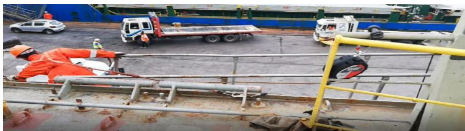
Figure 10d – Crew standing on the lower platform with the lifeline connected to the fall arrestor – (Source: UEIM video screen grab)
