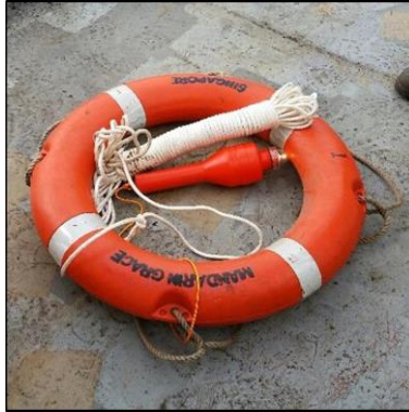
Figure 2 – Lifebuoy with self-igniting light and buoyant lifeline – (Source: UEİM 8 )
