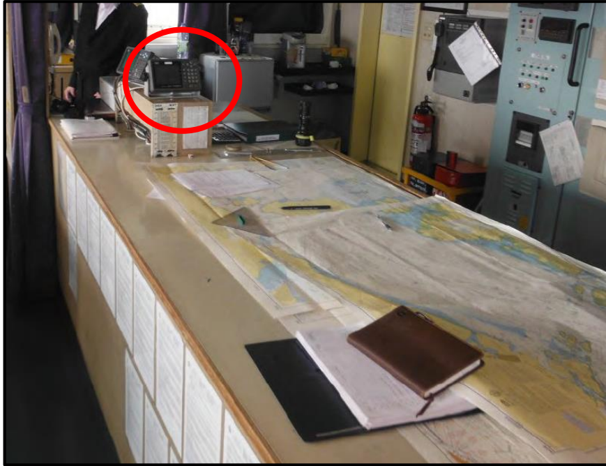
Figure 8: Chart table (separated by curtain in hours of darkness) on EP's bridge with AIS (circled red by TSIB) display equipment Source: LISCR
