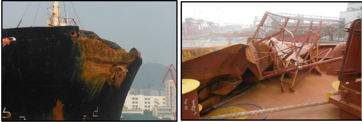
Figure 4: Damages on MV Eirini P's port bow. Source: LISCR
