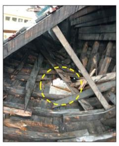
Figure 2 – WC's view from the outside and inside showing a hole on the port side
