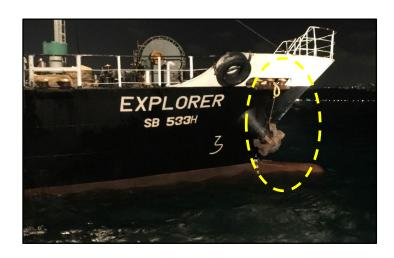
Figure 1 – The EXP's starboard bow with minor scratches – annotated by TSIB
