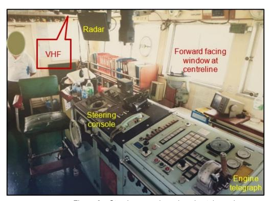
Figure 6 – Steering console and engine telegraph
