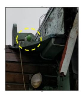
Figure 4 – Zero-watt green bulb on the starboard side - annotated by TSIB
