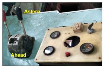
Figure 5 – Engine throttle position (annotated by TSIB)
