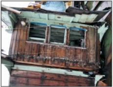
Figure 3 - The steering position (located at the aft end of the WC) and the three windows (viewed from front) facing forward for visual navigation
