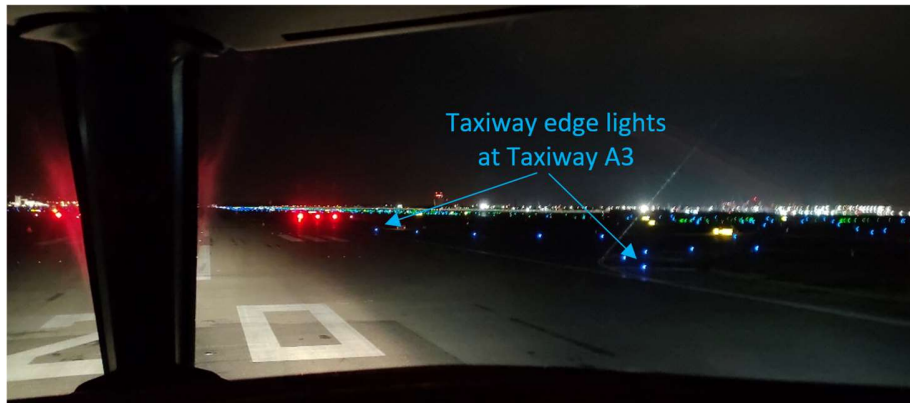
Figure 12: Taxiway edge lights, near the runway threshold, ON with runway edge lights OFF
