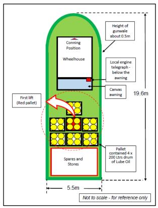
Fig.2 - Illustration of transfer plan
