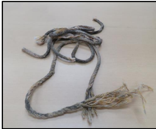
Figure 5 - The fragments of the seizing twine (Source: Ministry of Manpower)
