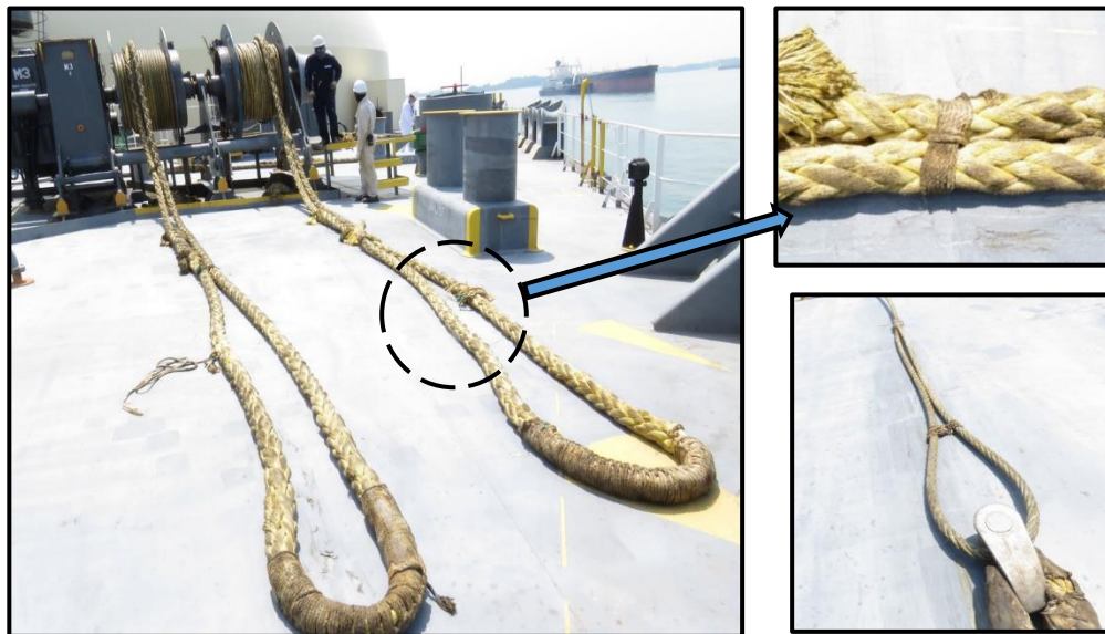
Figure 8 - An example of the original seizing on the tail end about 2.5m from the bight (top right) prior to it parting. Bottom right image shows tail's connection to the mooring wire via a tonsberg shackle (Source: Ministry of Manpower)
