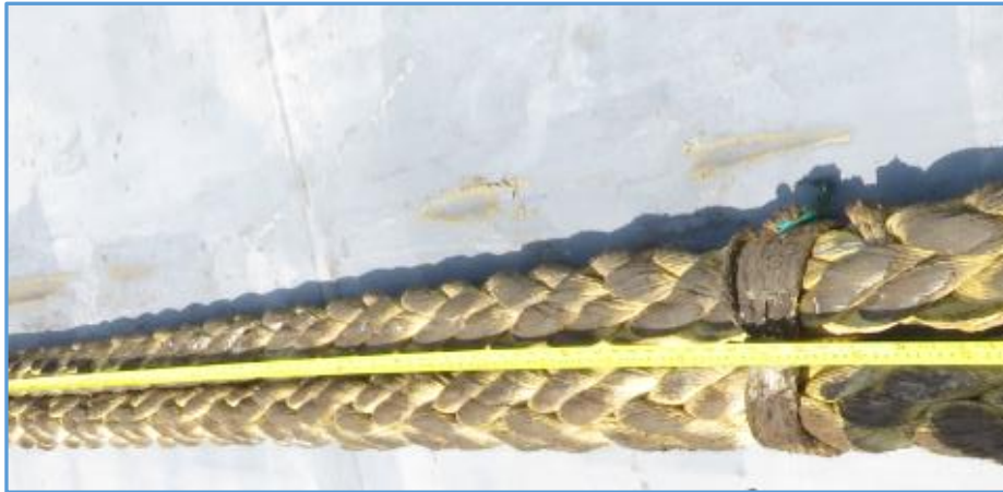
Figure 10 – Tail rope involved in at the time of the accident – Shown to indicate overall condition of the trope ( Source: Ministry of Manpower )
