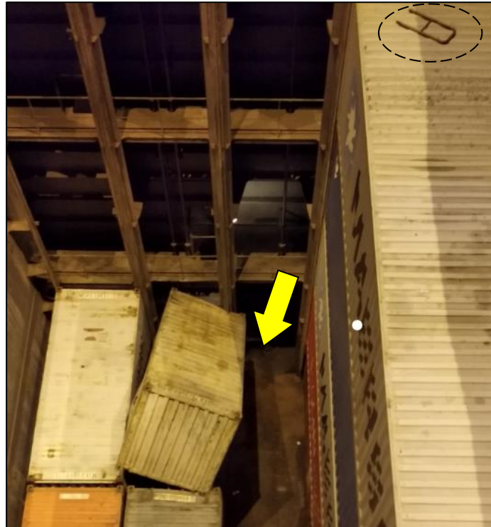
Figure 2: Photograph taken on site indicating the fallen container and the approximate location where the stevedore was found
