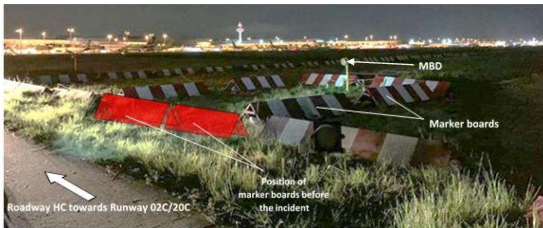
**Figure 5:** New marker boards positioned at roadway HC behind MBD.
