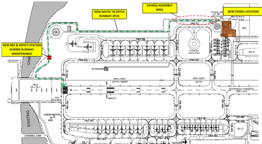
Figure 4: New route for entering and exiting the runway (indicated in green) and the new location of the store
