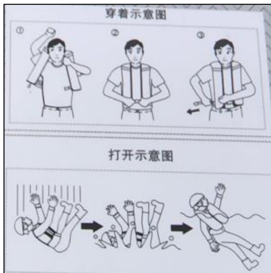
Figure 19 – Pictorial depiction of lifejacket's donning and operation.
