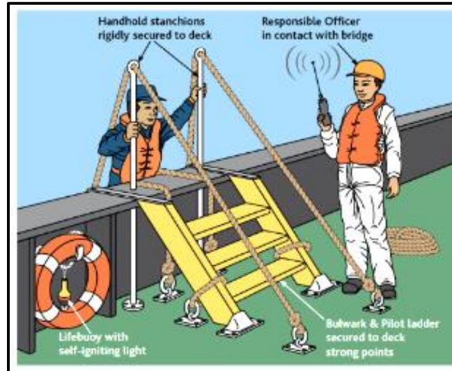
Figure 11: Boarding arrangement for safe pilot transfer with the need to climb over a bulwark or railing(s) to the deck. Source – IMPA.
